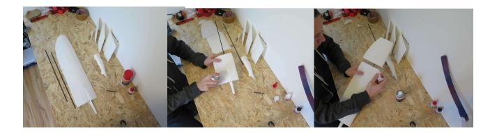
To assemble the wings, 2 carbon rods with a 4mm diameter are required (465mm for Floaterwing and 360mm for Acrowing). The assembly is explained here using the example of the floater wing, but works in exactly the same way for acrowing.
