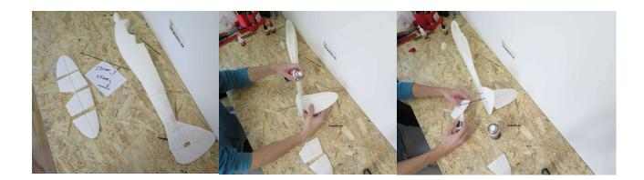
After the last part of HorStabL2 has been glued to the rest of the horizontal stabilizer, you can continue with the wings.
