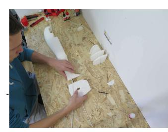
Next, connect VertStab to Fus4 - you need a carbon rod with a diameter of 3mm and a
