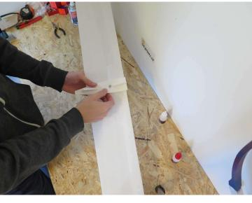
When everything fits, the carbon rod can be inserted into the Wingjoiner and the WingcenterL glued to the Wingjoiner - it is best to use thick superglue and apply it generously! Now the wing can be glued part by part on both sides, always making sure that the surface segments are flush.
