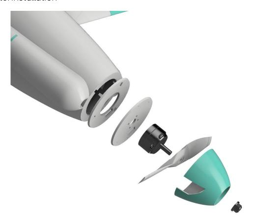
The "Motorplate" is glued to the "Fusefront" (pay attention to the teeth). Then, attach the motor to the "Motormount." The "Motormount" has 4 recesses for screws. Use a hot piece of piano wire to create corresponding holes in the "Motorplate," then secure the Motormount to the plate using small driver screws (e.g., servo mounting screws).
