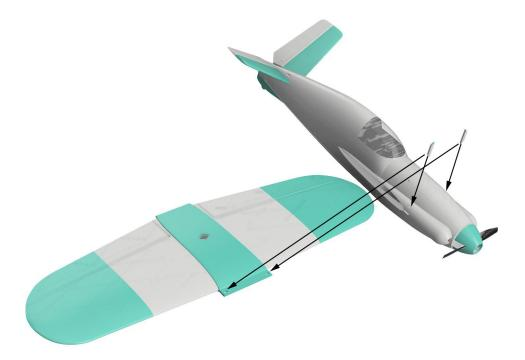
As previously mentioned, the wings can be permanently glued or designed to be removable. For better access in case of servo damage, a removable option is advantageous.
