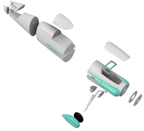
Glue Fusefront with Fuserear 1+2 - use 1 & 2mm carbon rods as guiding rails.
