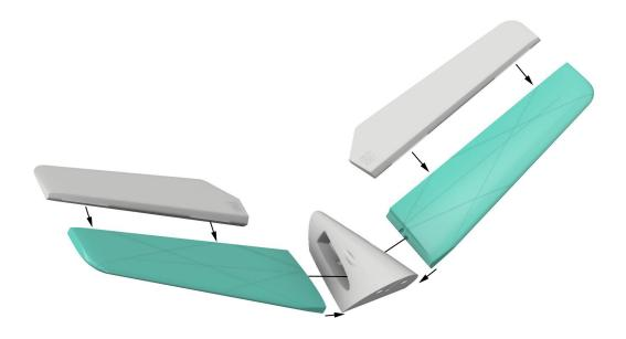
Check the fit of the 4mm carbon tubes and trim if necessary. Insert the tubes into VL and VR, and check the fit of the tail halves in the provided recesses. Then glue the tail halves together using medium-viscosity super glue.
